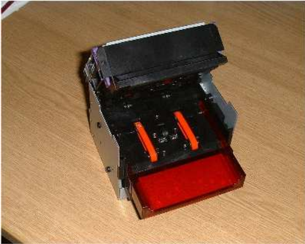
GBA HR1 in open position for cleaning and Jam Clearance.
